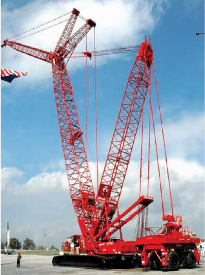
A high-efficiency, high-capacity, 400-ton crawler, the Manitowoc Model 16000 has many performance features that make it a workhorse contractor's crane as well as a rigger's crane.
