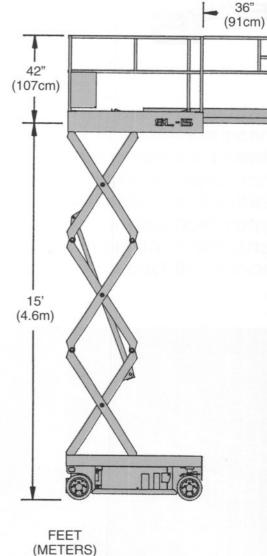
DANGER: Models described in this brochure are NON-INSULATED and do not provide electrocution protection from contact with or close proximity to energized conductors which is pointed out on decals and placards attached to the machine.
